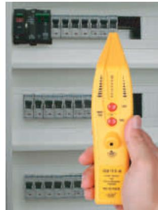
The Circuit breaker which supply the Transmitter circuitry is the one, which, when pointed out by the tip, has the most LEDs lit on the bar-graph and the fastest buzz.
